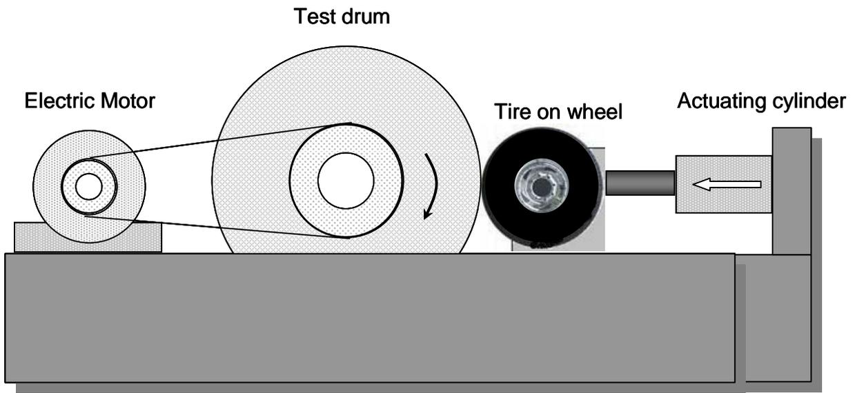
**Figure 4. Typical Test Configuration for Rolling Resistance Measurements**
